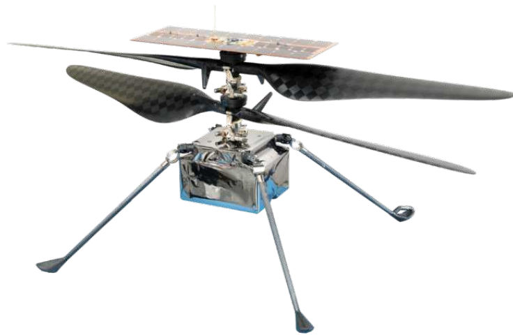
FIGURE 3. Ingenuity Mars Helicopter [6].
